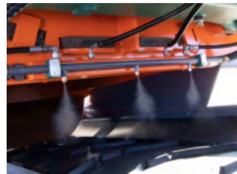
Water Sprinkler System
