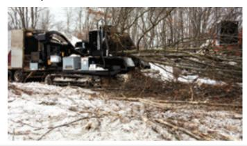
The Model 3090 Track comes standard with a Caterpillar steel track undercarriage. This feature allows it to travel over rough terrain not accessible by towable units. It also eliminates the need to forward or skid material to the chipper – the operator can take the chipper to the trees
