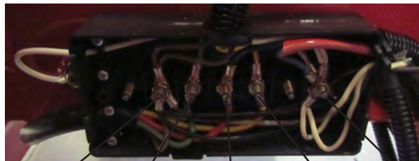
Running Lights (BR) Right Turn (G) Brakes (R) Left Turn (Y) Ground (W)
